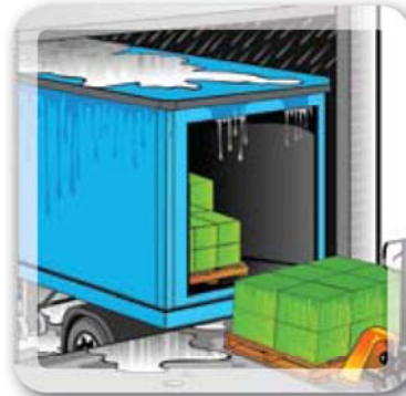
Water infiltration onto the loading dock area can lead to wet & slippery floors which can be dangerous to personnel.
